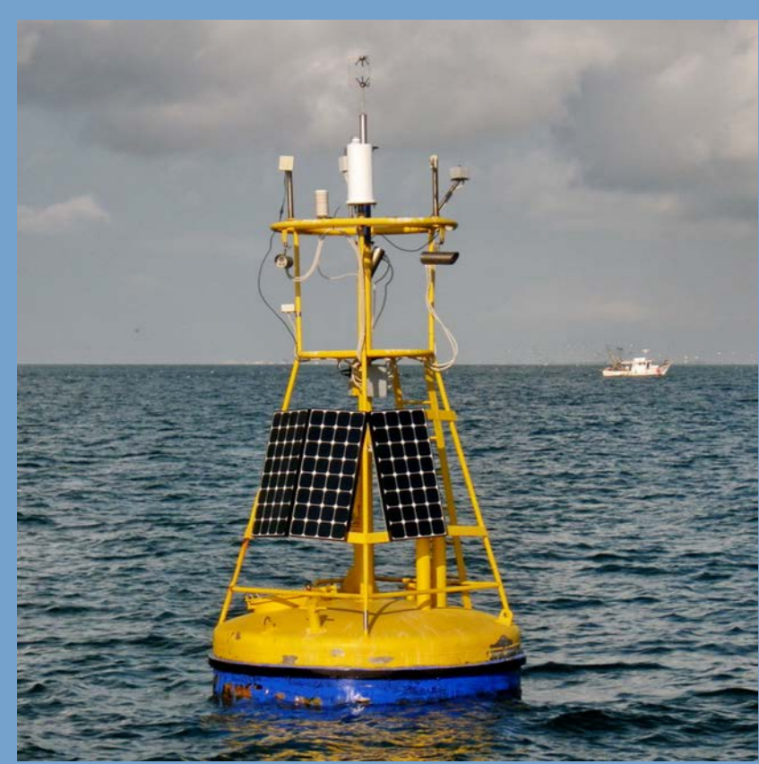
Figure 1: Oceanographic buoy Vida is continuously collecting oceanographic and meteorological data.
