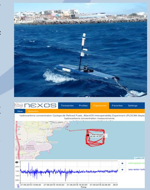
Within the **NeXOS project** two PUCK-enabled sensors (Mini.1 Hydrocarbons detector and Smart Hydrophone A1) were deployed in a SeaExplorer
