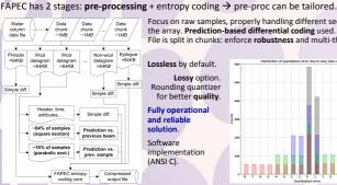
Focus on raw samples, properly handling different sections of
