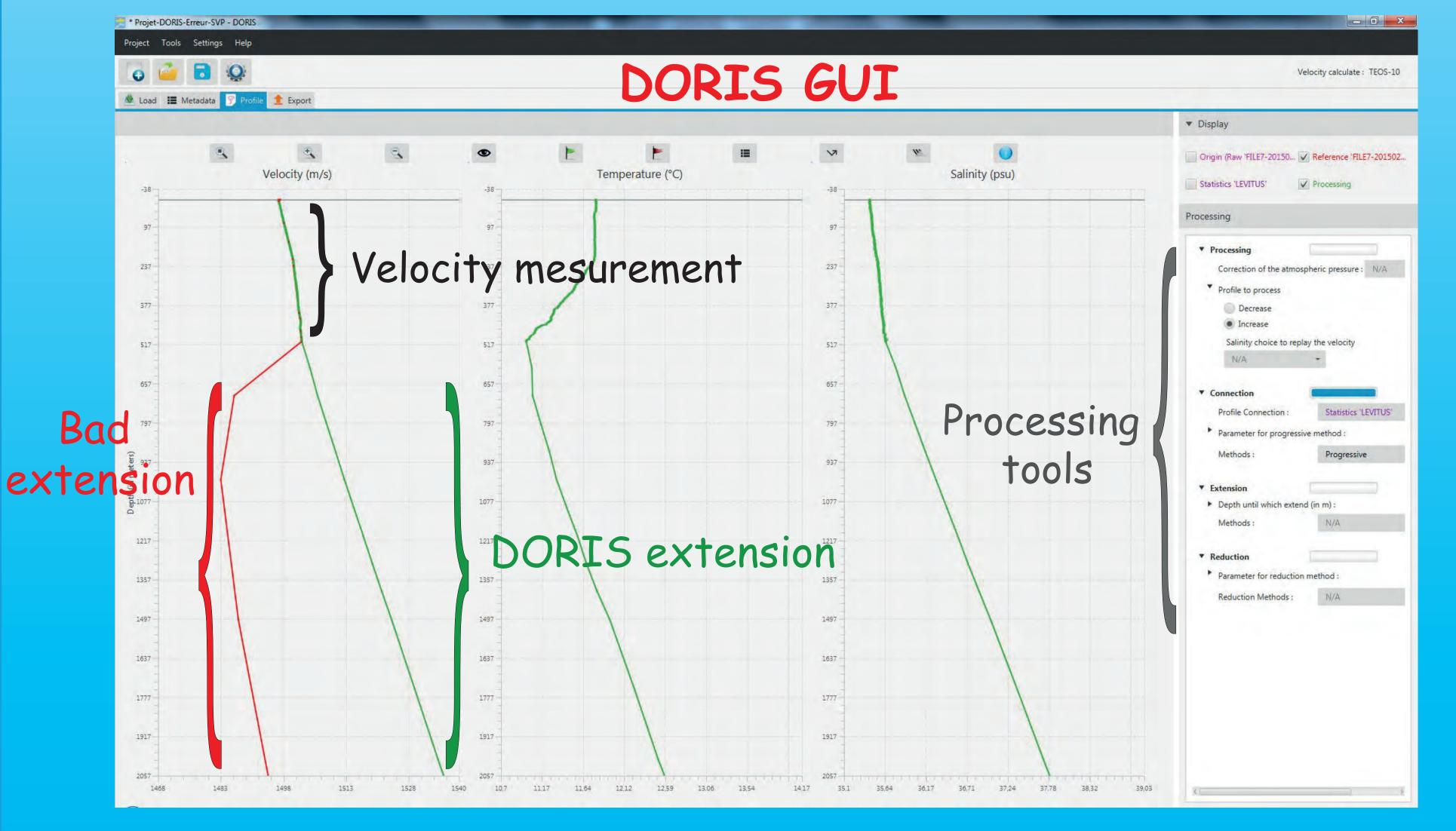
Data uploading from sound velocity sensors
