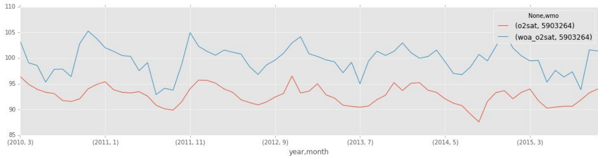
Fig. 2 – Over 5 years of surface oxygen saturation measured by Bio-Argo float 5903264 (blue) compared with oxygen saturation from the World Ocean Atlas (red). The biofloat Python software enabled easy generation of this plot in a Jupyter Notebook.
